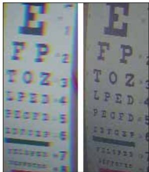
Gulden says viewing eye charts through new Correct-a-Prizm and Correct-a-Prizmbar significantly reduces chromatic aberration seen by a patient, improving his or her ability to discern charts resulting in more accurate examination and diagnosis. Left view is without ComPrizm; right view is with ComPrizm.
